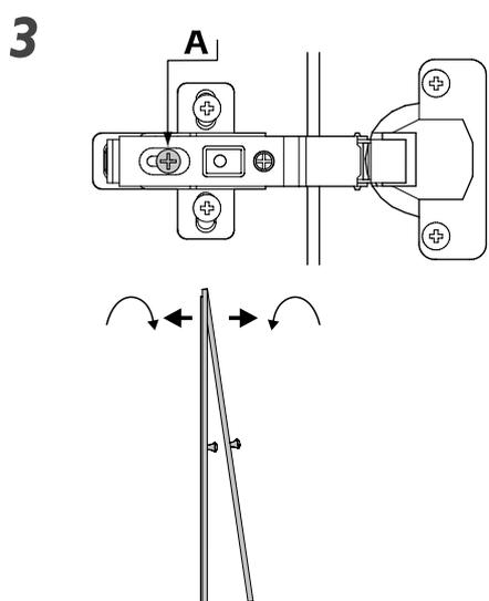
Adjusting the angle of the door. Loosen screw 'A' and slide the hinge arm either forwards or backwards until the door is vertical then tighten screw 'A'.
