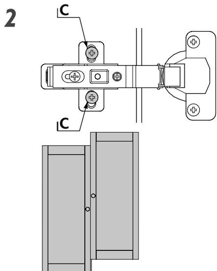
Adjusting the height of the doors. Loosen screws 'C' then slide the hingeplates up or down until the doors are even then tighten the screws.
