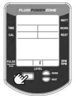
Turn handle to Level 1. Press Reset. Display will now show Level 2. Level 1 Calibration is complete.
