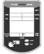
Turn handle to Level 2. Press Reset. Display will now show Level 3. Level 2 Calibration is complete.
