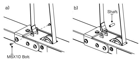
Hold the Belt. Remove 2x M6x10mm Bolt and the Shaft.
