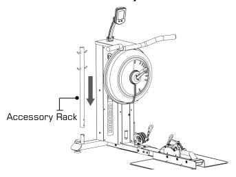
b) Secure using 4x M6x15mm Bolt [8]
