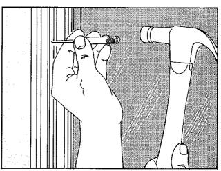
8. Reset inside stops starting with the sides, driving nails in the same holes at different angles.
