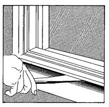
2. Pry stops loose with wide spatula, then remove being careful to prevent breakage and marring inside finish.
