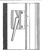
12. Insert perforated points of template in screw holes of keeper. Engage keeper in sash lock and lock.
