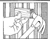
14. After keepers are installed check for proper operation. It may be necessary to relocate the inside stop if binding occurs on hinge side of sash. Inside stop is moved by first breaking paint or varnish
