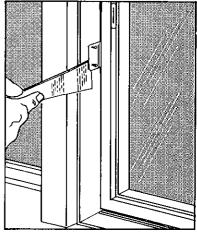
4. Loosen stationary sash clips from frame and remove sash.
