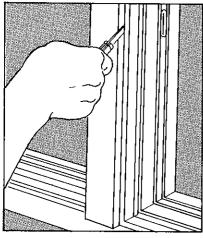
1. Carefully remove top and bottom stops by first breaking paint or varnish seal with a sharp pen knife or spatula.
