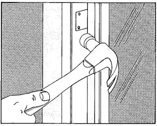
6. Nail sash clips to frame making sure sash fits snugly against the frame.
