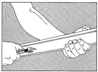
7. Pull nails through rather than back out on removed stops. This will eliminate any chipping on face side of stops.
