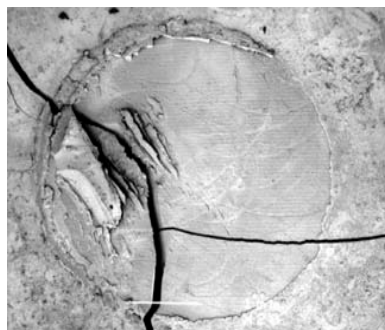
Figure 7. Representative mixed adhesive-cohesive failure on the surface of dentin after composite is debonded under shear loading (237 N).
