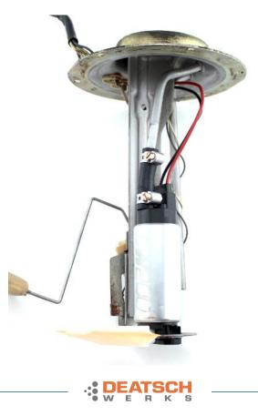
6 – reinstall the assembly into the fuel tank and attach a length of hose to the outlet of the pump assembly allowing it to drain into a fuel safe container and prime the fuel pump assembly
