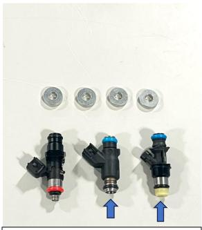
Factory LM7, LQ9, L92 Truck Injector examples next to the "Mid" height Injector from this kit.
