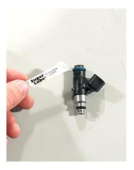
2C. Install the Short Adapters onto the tops of all your injectors as shown.
