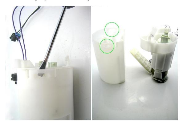
5 – remove the OE fuel pump by squeezing the tabs and pulling the pump away from the center assembly
