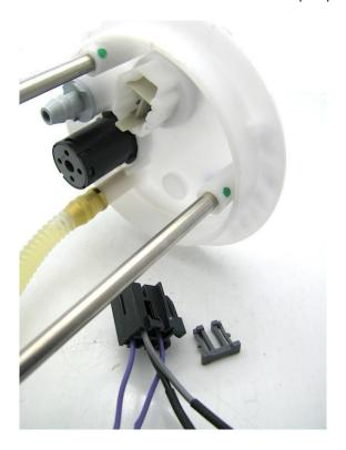
2 – carefully remove the tube connecting the fuel pump the fuel pump assembly, by cutting it with a sharp knife
