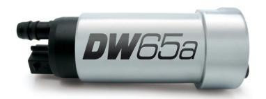
The DW65a in-tank fuel pump with install kit was specifically designed for the Holden Commodore Gen III 97-06 5.7/6.0 V8 but also fits other popular applications (see application guide). The DW65a flows 265lph at 40psi and features a quiet and reliable turbine impeller which is compatible with pulse width modulated pump drivers. The pump also features an encapsulated armature for compatibility with ethanol based fuels. All DW fuel pumps are backed by a 3-yr no fault warranty.
