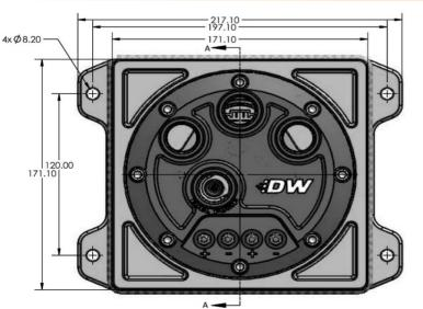
DW's staged surge tank is engineered to provide massive amounts of fuel flow reliably and consistently for racing applications. The DW 5.5 Liter Staged Surge Tank System includes the functionality of traditional surge tanks, with increased flexibility. This has been achieved by moving the pumps inside with a merged single point outlet that allows the use of single, dual, or triple pump configurations to meet fueling needs from 500hp to 2000hp
