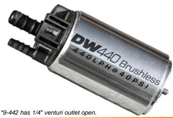
The DW440 brings brushless pump technology INTO the fuel tank. With a total height of only 4 inches (103mm), it is the only highflow aftermarket brushless pump that is easily retro-fitted into an OE pump module. Brushless technology reduces friction and heat, increases effeciency, vastly improves pump lifespan in ethanol and methanol fuels, and allows higher voltage inputs for increased flow.
