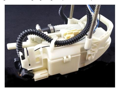
9 – reinstall the assembly into the fuel tank and attach a length of hose to the outlet of the pump assembly allowing it to drain into a fuel safe container and prime the fuel pump assembly
