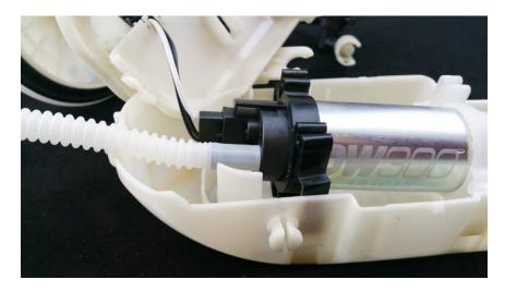
7 – remove the assembly inlet (line from pump outlet) by gently pulling out, attach the rubber hose on the end of the preinstalled plastic hose on the pump to the assembly inlet, then replace after tightening hose clamp
