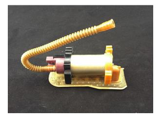
5 – transfer the OE filter and front support to the DW200/300
