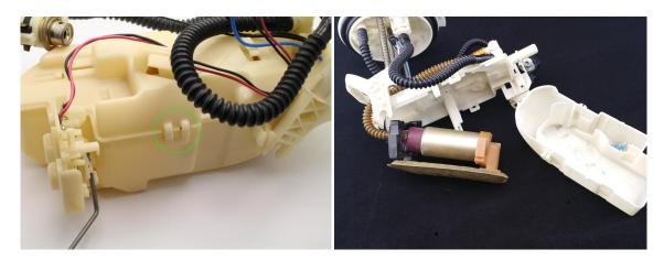
4- disconnect the fuel supply line from the assembly with a sharp hobby style knife, remove the fuel filter and the front support. These will transfer to the DW200/300
