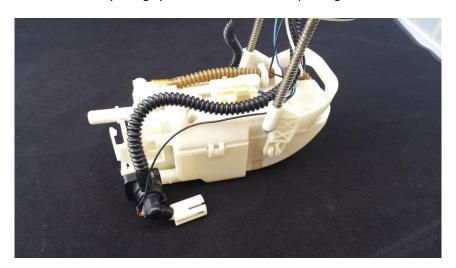
2 – remove wires from their holders and separate the top hat from the assembly by pulling up
