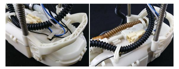
1 – disconnect the return line by lifting up the tab on the side and pushing down the tab on the front
