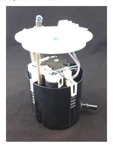
10 – reinstall the assembly into the fuel tank and attach a length of hose to the outlet of the pump assembly allowing it to drain into a fuel safe container and prime the fuel pump assembly
