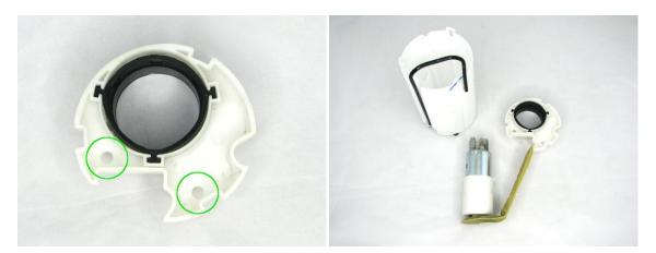
4 – insert the DW400 into the center section, install the pump fuel sock, and clock like pictured below and install into the bucket assembly. Push center section down until it clicks in place below the ridges in the bucket assembly:
