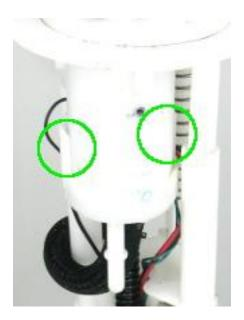
6 – before reinstalling the hat assembly into the center/bucket assembly, push both the 3/8" pump outlet hose and tighten the hose clamp and push on the 1/8" venturi feed hose and crimp the 1/8" permanent clamp in place using dykes or side cutters. Now push hat assembly into the center/bucket assembly and push the pump outlet tube onto the hat assembly
