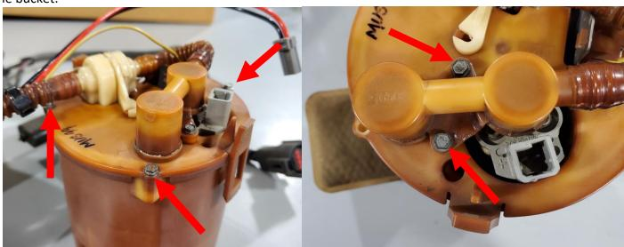
2 – Separate the pump outlet from the lid by lifting, the lid bucket and pump seal onto internal O-rings, take care when prying up not to damage the O-rings or the plastic. Remove the lid from the bucket once the pump outlet is removed.
