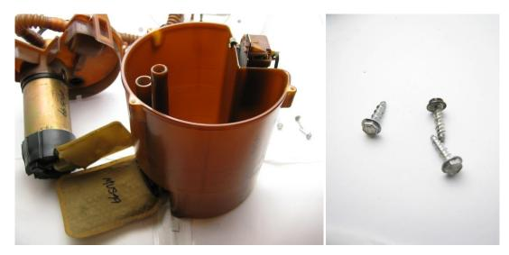
2 - remove the OE sock and isolator from the OE pump and install on the DW300m
