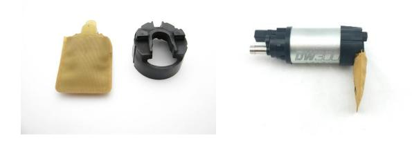
3 - remove the OE sock from the bucket and install the new sock supplied in the kit
