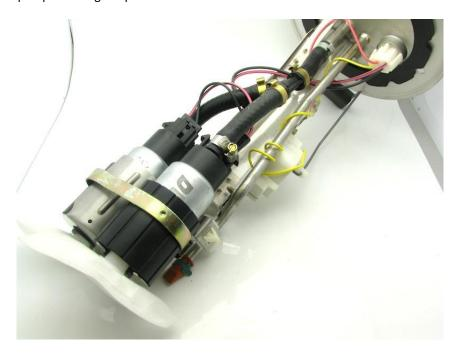
6 – reinstall the assembly into the fuel tank and attach a length of hose to the outlet of the pump assembly allowing it to drain into a fuel safe container and prime the fuel pump assembly
