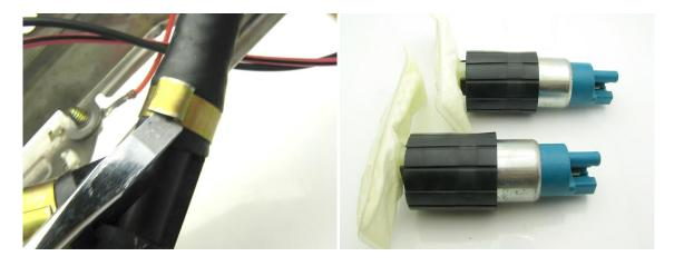
3 – reuse the pump isolators and install the fuel sock and sock retainer
