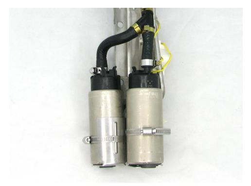
6 – install the fuel socks onto the bottoms of the DW400s
