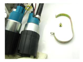
2 – loosen the OE hose clamps from both pumps and remove the pumps. Remove the upper hose clamps and remove the OE hose (it may need to be cut to remove, careful to not score the barbs underneath). Install the supplied DW hose, the longer hose goes on to the angled inlet
