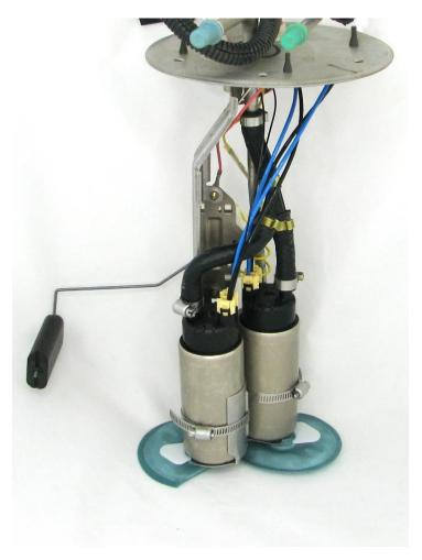
8 – reinstall the assembly into the fuel tank and attach a length of hose to the outlet of the pump assembly allowing it to drain into a fuel safe container and prime the fuel pump assembly
