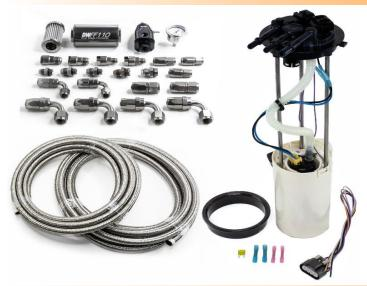
The DW400 99-04 GM Truck Module is a complete plug-nplay replacement for the OE unit. The module incorporates the DW400 pump which more than doubles the flow output of the OE module. This module also integrates seamlessly with the OE wiring harness and level sender. The module includes a return plumbing kit with 8AN feed and 6AN return lines, a DWR1000 regulator, fuel pressure gauge, and DW 110mm 10-micron stainless steel fuel filter.
