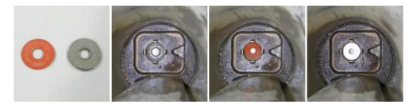
4 – assembly the pump pre-filter kit (fuel sock and grommet) and install onto the DW65c pump
