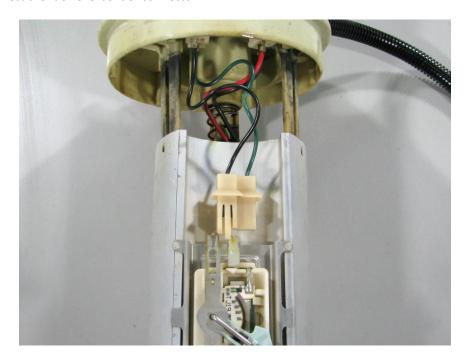
2 – separate the pump assembly from the bucket by depressing the 3 vertical supports while pulling the assembly hat away from the bucket
