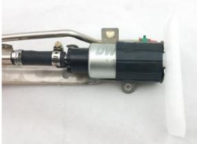
5 – install the pump retaining strap
