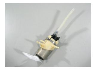
4 – wire in the supplied electrical connector (blue-to-red and black-to-brown, the additional smaller black lead can be removed) and push the PTFE hose onto the assembly inlet. Secure the pump in place using the OE rubber isolators
