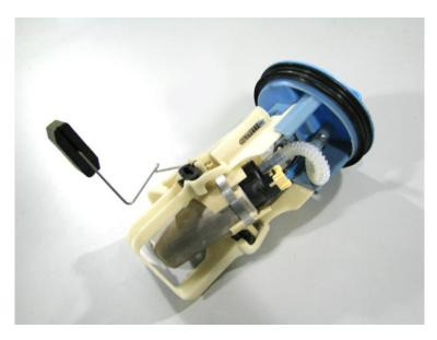
5 – adjust the height of the pump in the pump holder until the pre-filter is near the bottom of the assembly, and tighten the large hose clamp. Do Not Overtighten – pump damage can occur.
