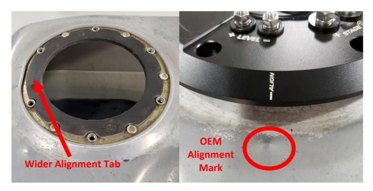
16 – Install and tighten the provided mounting bolts to the factory torque spec.
