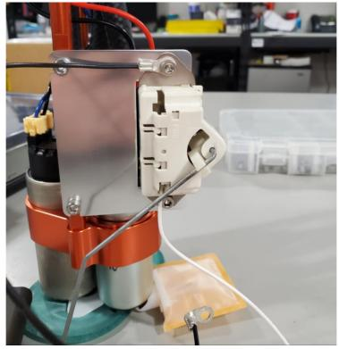
8 – Attach the 90-degree ring terminal ends of the level sensor ground and signal wires to the module. The ground should attach to the Level – (Negative) terminal and the signal wire to the Level + (Positive) terminal.
