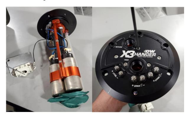
12 – Install the module into the fuel tank; slip the fuel level sensor in first, followed by the module. Remove the remaining 2 module bolts and sit the top plate out of the way.
