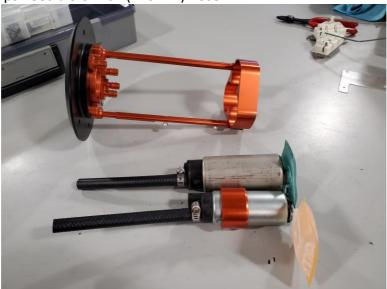
2 – Install the pumps into the module, if you are using a 39mm pump (DW100, 200 or 300) you will need to install the supplied adapter sleeve onto the pump body before installing it into the pump holder.
