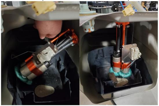
14 – Orientate and reattach the top plate to the module hanger, be careful that all the O-rings stay in place, this may require lifting the hanger portion back up out of the tank while tightening. Re-connect any pump wiring you unhooked during install. Once fully installed inspect the convoluted return hose and make sure it is still directed into the black tub inside the fuel tank.
