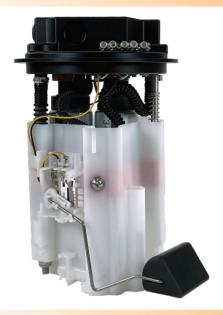
The new DeatschWerks X2-Series Subaru Module is now available for the 2008-21 model years, which includes accommodation for 2 pumps, integration of a return fuel line, and retention of ALL the functionality of OE module. The DW X2-Series Subaru Module consists of a top-hat, center section, and OE lower bucket. These 3 components work together to deliver the flow you need and the OE functionality you want.
