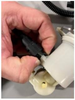
2 – Remove the OE fuel hose from the OE EFI fitting (yellow arrow). Remove the small OE venturi hose located on the side of the lower fuel pump assembly on the brass hose barb fitting (red arrow). Using a razor blade carefully cut a small slit on both hoses without damaging any of the parts you are removing the hoses from (blue arrow). You will be reusing the OE EFI fuel fitting.
