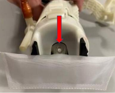
8 – Install the other end of the venturi hose. Preinstall a small permanent clamp onto the hose then slide the hose onto the OE brass fitting located on the side of the lower fuel pump. Make sure the hose is slid all the way onto the hose barb until it bottoms out. Squeeze the permanent clamp tight using crimpers or side cutters (picture below).
