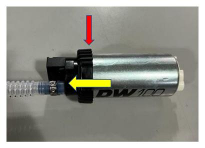
6 – Install the small venturi hose onto the venturi hose barb located on the top of the DW fuel pump. Preinstall one of the smallest permanent clamps onto the hose. Pressing firmly install this end of the hose onto the venturi hose barb until the hose bottoms out on the hose barbs base. Align the small clamp in the direction shown below (red arrow) make sure the clamp is all the way to the bottom of the installed hose. Squeeze the permanent clamp tight using crimpers or side cutters.
