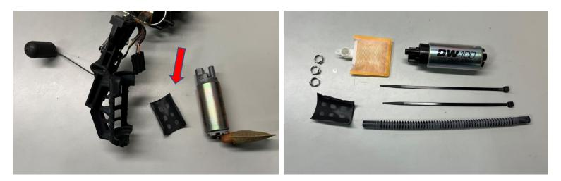
4 –Install the supplied filter sock onto the DW fuel pump. Recommend using a small screwdriver or a small socket to press the lock washer on the filter stud until it is fully seated (red arrow).
