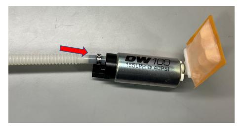
6 – Install the OE rubber isolator on the back of the DW fuel pump. Place the pump with the isolator against the fuel pump assembly (yellow arrow). Install the supplied (2) zip ties around the pump assembly bracket and the DW fuel pump (red arrows). Verify the zip ties are tightened fully. Cut the ends of the zip ties off using a pair of side cutters for cleaner appearance and better fitment into the tank.
