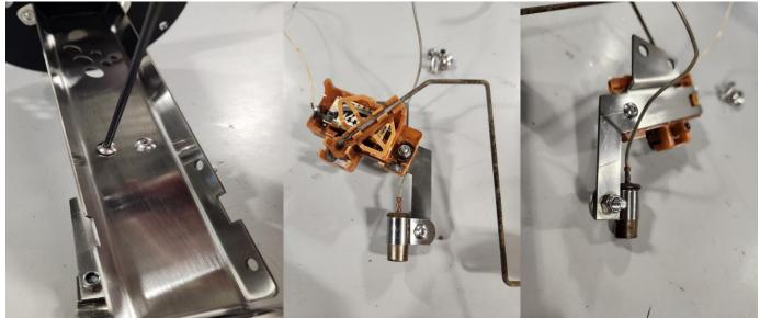
4 –Strip the ends of both wires carefully and crimp on the supplied 18-22awg ring terminals. Bolt the fuel level sensor assembly back to the main hanger bracket, it may be necessary to leave some bolts loose and retighten once everything is assembled. You can now attach the ring terminals to their respective terminals. The small metal canister wire should go to "Light+" and the level float sensor goes to "Level+", both sensors are grounded through the body of the hanger assembly.
