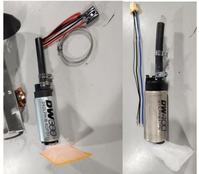
8 – Install the pumps into the hanger assembly, the filter sock will point the same direction as the fuel level float arm, this is important for fitment into the fuel tank. The pump is secured to the hanger assembly with the large 2-1/4" hose clamp, there are notches in the hanger to locate the clamp. Tighten the larger and small hose clamps.
