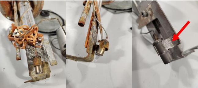
2 – You will also be reusing the OEM wiring harness for the level sensor, low fuel light and ground, as well as the fuel pump (if low amperage). Take a picture for future reference of the color and placement of the OEM wiring, then remove the OE wiring. The wiring color changes depending on year make and model.
