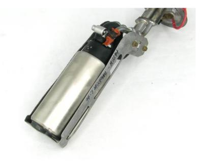
7 – install the fuel sock and wire in the electrical connector (blue is positive, the extra negative lead can be clipped or mounted to the assembly as an additional ground)
