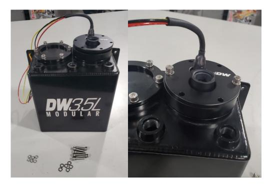
6 – Tighten the bolts in a star pattern to 30 inch/lbs.
