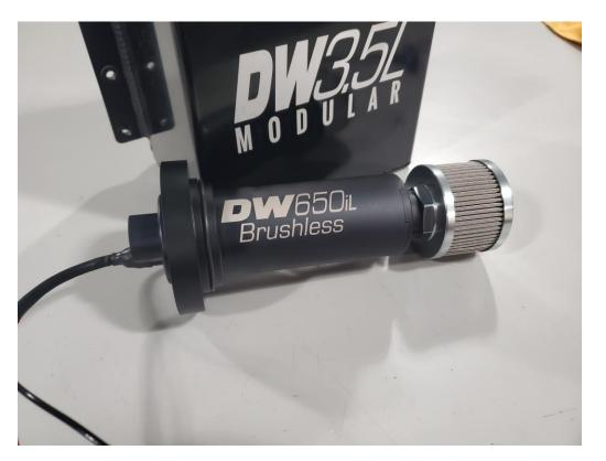
4 – Install the whole pump and adapter assembly into the surge tank. Slip the wiring harness through the top plate and locate the plate on top of the DW650iL pump, the opening is specific and can only slide over the pump one way.
