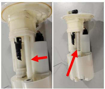
9 – Make sure to plug in the level sender and pump if you unplugged them. With this you are done with the module, and it is ready for installation into the vehicle.
