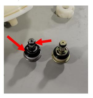
7 – Install the DW Performance In-Tank Regulator into the regulator port. Reinstall The regulator retainer. Make sure each tab is securely snapped onto the center section. This does see full fuel pressure.
