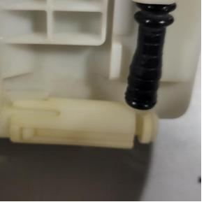
10 – Make sure to plug in the level sender and pump if you unplugged them. With this you are done with the module, and it is ready for installation into the vehicle.
