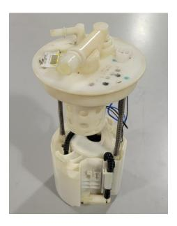
2 – Remove the top and center section from the bucket by undoing each locking tab. There are 3 on the bucket and 1 that is a part of the self-fill function. See the 3<sup>rd</sup> picture below.
