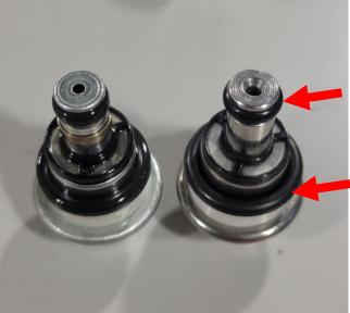
7 – Install the DW Performance In-Tank Regulator into the regulator port. Place the static discharge ground over the regulator prior to installing the retainer. If you do not have this piece skip that step. Reinstall The regulator retainer. Make sure each tab is securely snapped onto the center section. This does see full fuel pressure.
