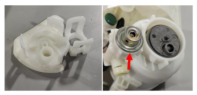
6 – Remove the factory regulator with a pick or screwdriver and place it to the side so it does not get mixed up with the DW Performance In-Tank Regulator. Place some lubrication on the regulators o-rings to ease installation. Shown in 2<sup>nd</sup> picture.
