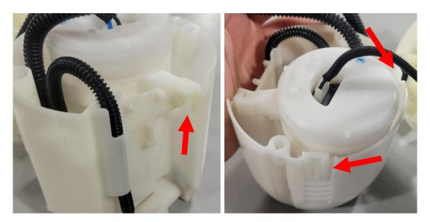
4 – The center section is now out. This will give you access to both the pump and the regulator.
