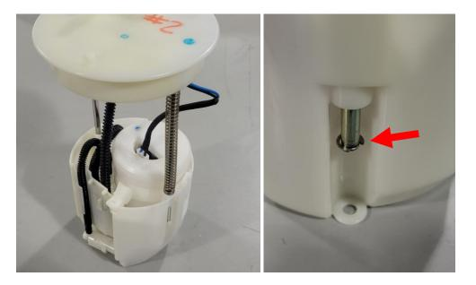
10 – Make sure to plug in the level sender and pump if you unplugged them. With this you are done with the module, and it is ready for installation into the vehicle.
