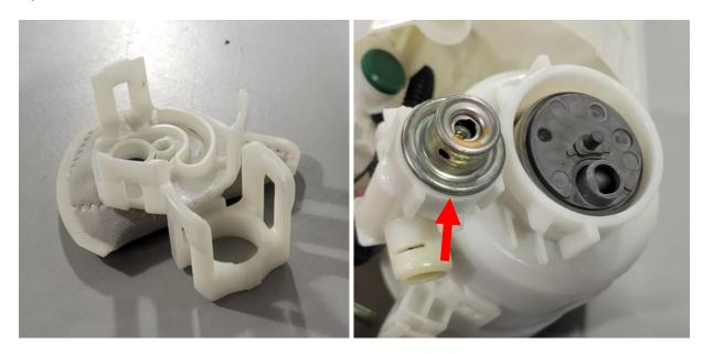
6 – Remove the factory regulator with a pick or screwdriver and place it to the side so it does not get mixed up with the DW Performance In-Tank Regulator. Place some lubrication on the regulators o-rings to ease installation. Shown in 2<sup>nd</sup> picture.
