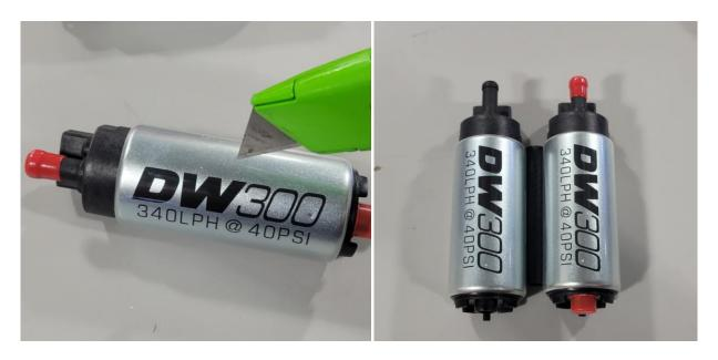
6a — We will now be installing the feeder pump. This pump will go into the slot that is all the way through the surge tank. Install the supplied pre-filter onto the inlet of the pump. Slot the pump into the empty hole from the bottom allowing the filter to slightly stick out. We want this pump to be the lowest in the tank to make sure it can keep the surge tank always supplied with fuel.
