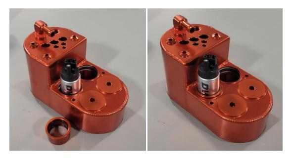
8a – We will now be installing the pressure pumps. Grab another one of your DW100/200/300 pumps and install the filter sock. Grab an additional 39mm pump adapter sleeve. Pre-install the sleeve onto the pump this time shown like in the  $2^{nd}$  picture. You will need to install the pump at an angle to get the filter sock into the surge tank.
