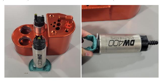
8b – You will need to pinch the filter and install at an angle like so. You can remove the lower o-ring in the surge tank to make installation easier. You may need to rotate and push the filter to get it into place.
