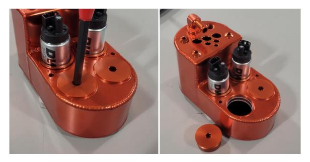
11a – If you are going to be running less than 3 pressure pumps, be sure to remove the corresponding nipple and block off that port. If you do not have any -6 AN ORB plugs (DW# 6-02-0717) you can use ones from the top of the surge tank. This will not hurt anything as the holes on the top are to allow for overflow from the tank. You will need a 1/4"Allen wrench to remove the plugs.
