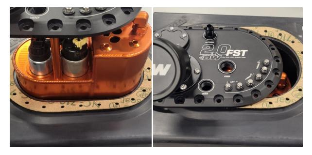
33 – Once the assembly is in. Slide over while keep the gasket held in place. Line up the bolts and you can use our supplied Allen head bolts or the ones that come with the tank. Install each bolt in a star pattern torquing in steps.
