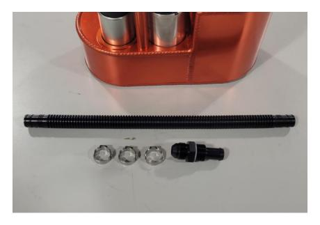
29 – Install the fitting into the top hat like so. Tighten down and the barb should protrude from the bottom of the top hat. Take the 1/2" hose and slip it over the Barb on the back of the sure tank. You do not need to install the clamps first as they can slide over the whole hose.
