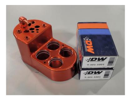
4b – Remove the pump and install kit from the box. It's best to do this one at a time to avoid losing parts. You will be not using one of the hoses supplied. One is 3/8" and the other is 5/16". You will only be using the 3/8 hose.
