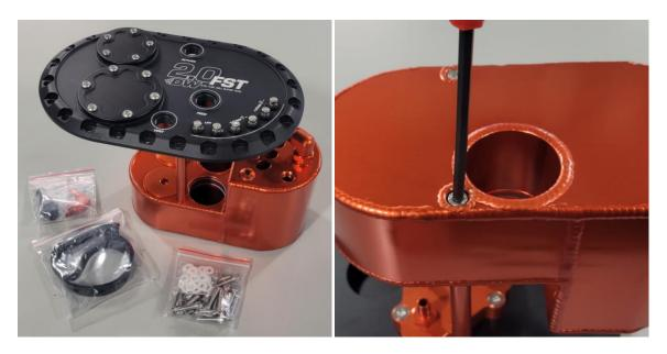
2 – Here is the surge tank and the top hat assembly disassembled. You do not have to remove the support rods for install. Place the surge tank mounting bolts to the side in a container for safe keeping as those will not be needed until the last couple steps.
