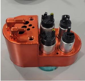
13 – Because the DW400 pump has a 3/8" outlet, we have included two different hoses for the feed pump. One hose is 3/8" on both sides use this hose for the DW400 feed pump applications, and the other longer hose is 3/8" on one side and 5/16" on the other, use this hose for DW100, 200 or 300 applications. Use the 5/16" end on the pump and the 3/8" side on the return fitting.
