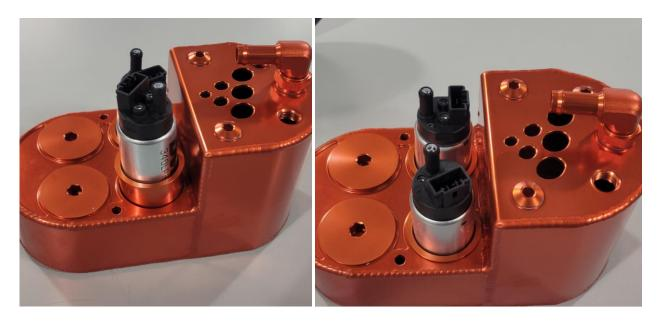
10a – Temporarily install the top hat and verify the pumps are aligned with their corresponding nipple. If not spin the pumps until they line up. This will make installing the hoses easier.
