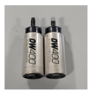
6b – Install the pump pre-filter on the feeder pump, then slot the pump into the bottom of the surge tank. Push the tank all the way down the pump until the sock is seated at the bottom of the tank.
