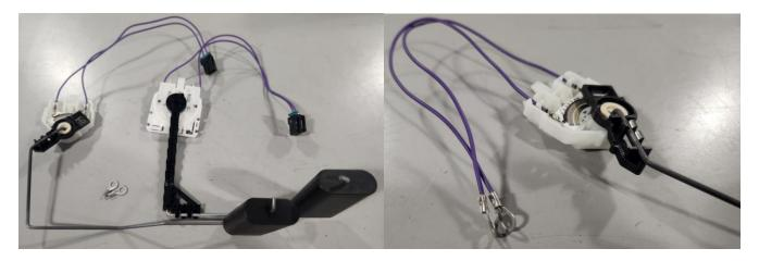
13 – Remove the M5 and M4 nuts and lock washers from the bottom side of the tophat assembly. Attach the Positive and Negative wires for one of the pumps to the Stage1 terminals. Attach both remaining Positive and Negative wires to the Stage2 terminals. This will allow you to run on one pump while cruising and turn on the remaining two pumps when you need them. Attach the two fuel level sending unit wires to the Level Sensor terminals. Replace the lock washers and nuts, tighten appropriately.
