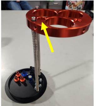
7 – Slide your pumps into the orange pump holder plate and attach the free end of your convoluted tubing to the three orange 3/8" hose barb fittings on the tophat assembly. Location does not matter since when all pumps merge into the same 10AN Feed port.
