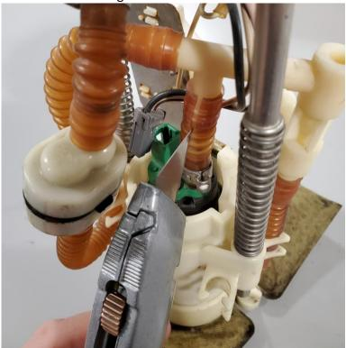
2 – Remove the two screws that hold the lower pump retainer onto the module, take care not to damage the ground wire for the level sending unit. Remove the pump, filter sock, hose and lower retainer from the rest of the module.
