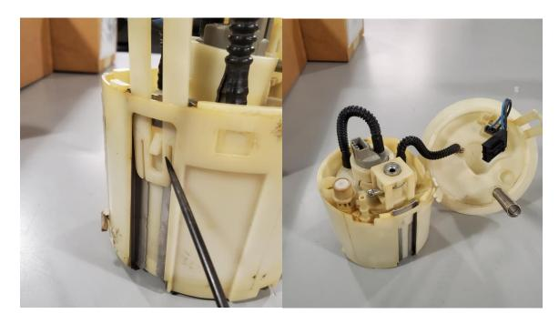
2 – Separate the filter center section from the bucket assembly, by gently prying the locking tabs away from the bucket. These can be brittle depending on the age of the module.
