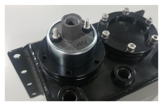
6 – Install Retaining ring on top of pump with the 6 retaining bolts and lock washers. \*Torque to 30 in/lbs.
