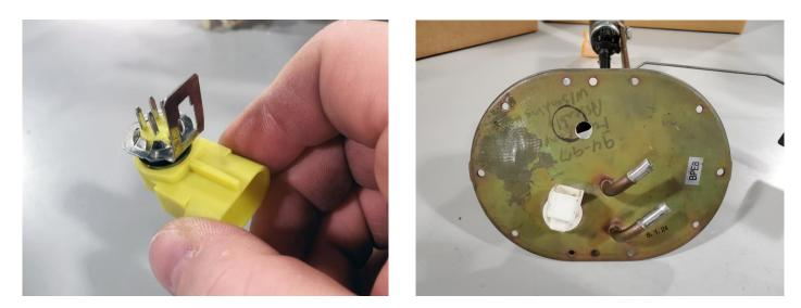
6 – The factory fuel pump power and ground wires can be removed or covered so they will not short on the module. Attach the supplied Brushless pump harness to the bulkhead and the DW440 pump.
