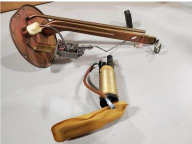
2 – Attach the supplied filter sock to the bottom of the DW Brushless fuel pump, secure the filter sock with the included star washer, this can sometimes be difficult to install, it can be made easier by using a socket to push evenly on the edges of the washer.
