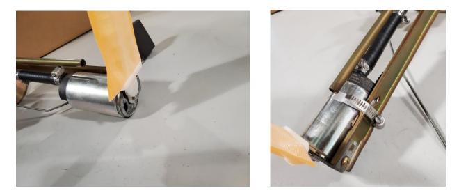
4 – Install the supplied fuel safe submersible rubber hose between the pump and the module, use the two supplied adjustable hose clamps to secure the hose in place. The supplied hose is 4 inches long, it may be cut down to fit as needed.
