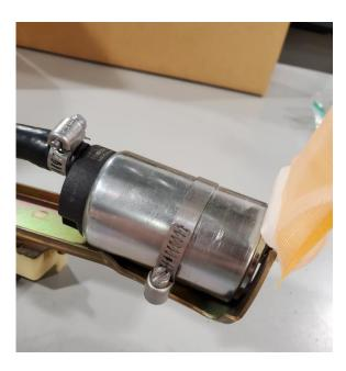
4 – Install the supplied fuel safe submersible rubber hose between the pump and the module, use the two supplied adjustable hose clamps to secure the hose in place. The supplied hose is 4 inches long, it may be cut down to fit as needed.
