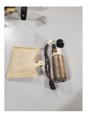
2 – Attach the supplied filter sock to the bottom of the DW Brushless fuel pump, secure the filter sock with the included star washer, this can often be a pain to install, it can be made easier by using a socket to push evenly on the edges of the washer.
