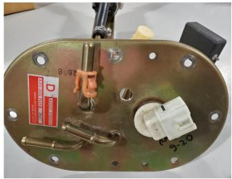
6 – The factory fuel pump power and ground wires can be removed or covered so they will not short on the module. Attach the supplied Brushless pump harness to the bulkhead and the DW440 pump.
