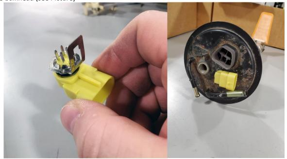
6 – The factory fuel pump power and ground wires can be removed or covered so they will not short on the module. Attach the supplied Brushless pump harness to the bulkhead and the DW440 pump.
