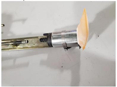
4 – Install the supplied fuel safe submersible rubber hose between the pump and the module, use the two supplied adjustable hose clamps to secure the hose in place. The supplied hose is 4 inches long, it may be cut down to fit as needed.
