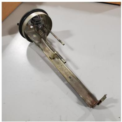
2 – Attach the supplied filter sock to the bottom of the DW Brushless fuel pump, secure the filter sock with the included star washer, this can often be a pain to install, it can be made easier by using a socket to push evenly on the edges of the washer.
