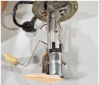
4 – Install the supplied fuel safe submersible rubber hose between the pump and the module, use the two supplied adjustable hose clamps to secure the hose in place. The supplied hose is 4 inches long, it may be cut down to fit as needed.
