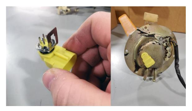
6 – The factory fuel pump power and ground wires can be removed or covered so they will not short on the module. Attach the supplied Brushless pump harness to the bulkhead and the DW440 pump.
