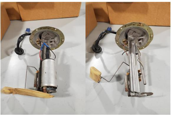
2 – Attach the supplied filter sock to the bottom of the DW Brushless fuel pump, secure the filter sock with the included star washer, this can often be a pain to install, it can be made easier by using a socket to push evenly on the edges of the washer.
