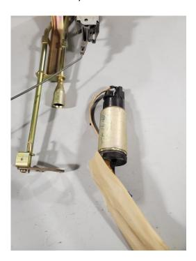
2 – Attach the supplied filter sock to the bottom of the DW Brushless fuel pump, secure the filter sock with the included star washer, this can often be a pain to install, it can be made easier by using a socket to push evenly on the edges of the washer.
