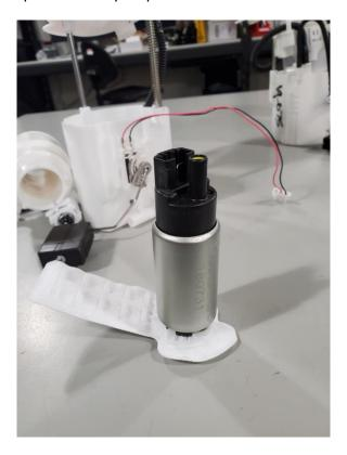
6 – Install the supplied O-rings on the pump outlet, you must use both O-rings, the bottom is a spacer to locate the top one at the correct height. Lubricate the O-rings with the supplied SuperLube prior to installation into the module.
