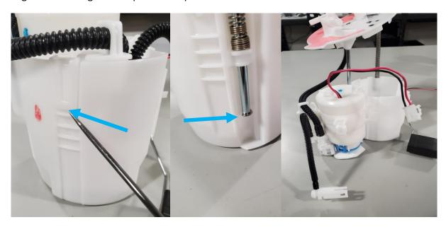
4 – Remove the factory fuel pump by unlatching the filter sock from the bottom of the filter center assembly. The pump may be held in place by the O-rings, you can push on the pump from the top connector side to remove it. Be sure to remove the O-ring from the center filter section if it remains in place and not on the pump.
