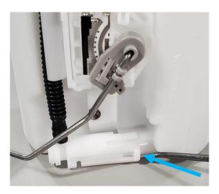
2 – Unplug the factory electrical connectors for the pump and sending unit, unclip the wires from their holders on the filter center assembly.
