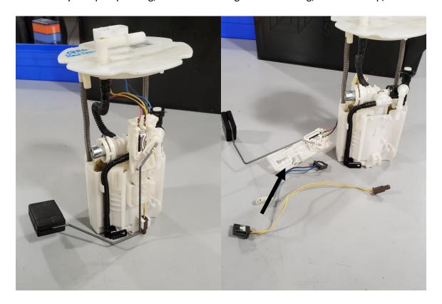
2 – Unhook the venturi hose connection from the side of the bucket, and compress and remove the plastic clip that holds the top hat to the bucket.
