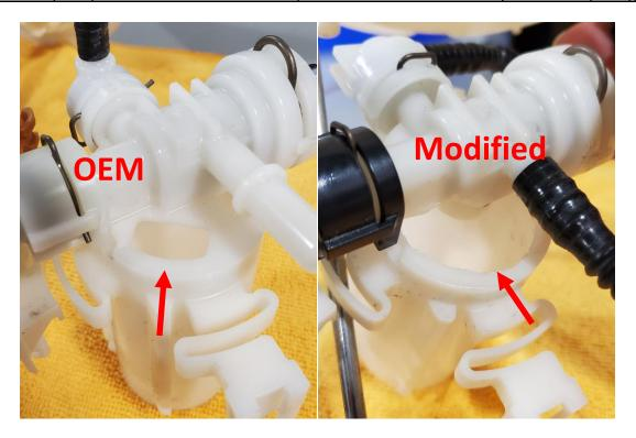
6 – Install the supplied spacer and O-rings onto the pump outlet, lubricate the O-rings with the supplied superlube. Install the supplied filter sock, make sure the alignment peg is inside the recess in the middle of the filter sock for correct alignment.
