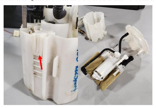
4 – Remove the factory fuel pump and filter sock, by lifting the two locking tabs on either side of the filter sock. Slide the pump out of the center section by pushing down on the connector area.
