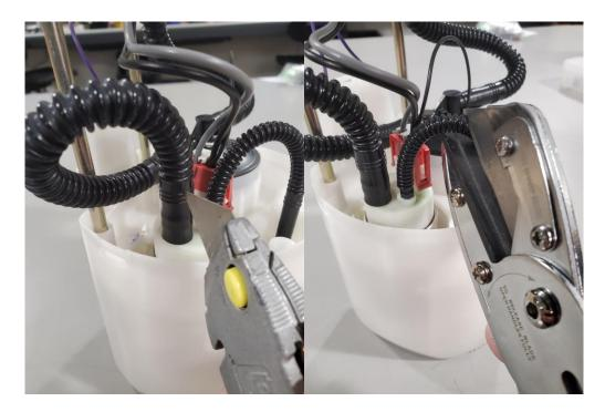
2 – Separate the bucket from the center section by unlatching the 3 clips around the edge of the bucket.
