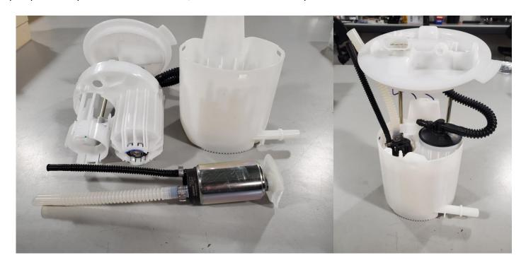
6 – Trim off the flare at the very end of the 1/4" venturi hose so you can apply the 7mm hose clamp over the hose. Attach the hose to the venturi jet inlet on the bucket and clamp with the 7mm clamp.
