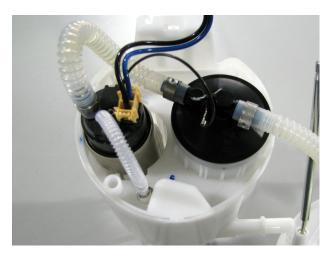
8 – reinstall the assembly top-hat to the center/buckets assemblies and connect the electrical connector harness to the hat assembly. Reinstall the fuel level sender and connector the electrical connector to the assembly top-hat
