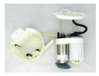
6 – install assembly center section into the assembly bucket and connect the 3/8" tube to the outlet of the pump, then pinch the 13.3mm permanent clamps. Slide the larger permanent clamp (7mm) onto the hose and crimp it in place (over the barbs) with a pair of side-cutters. Slide the smaller permanent clamp (6.1mm) on the hose and install the free end on the smaller venturi outlet on the pump. Crimp the clamp in place under the barb
