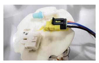
14 – Plug the 3-wire pigtail harness into the controller.
