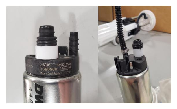
8 – Install the pump into the center section, all 3 of the O-rings should be seated inside the inlet of the module center section, lock the pump into place by latching the three lock tabs on the filter sock retainer. Slip the venturi hose into the OEM position, it should extend out of the center section. Connect the pump harness to the pump at this point.
