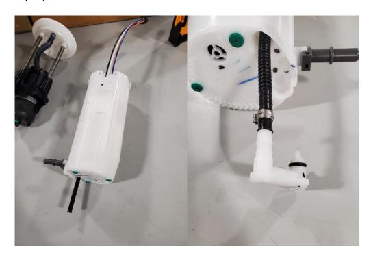
10 – Install the top hat section back onto the module, you will need to route the new brushless wiring between the filter and the black plastic retainer, if you run the wiring behind the fuel level sensor it will cause the float level arm to hang and give incorrect fuel level readings.
