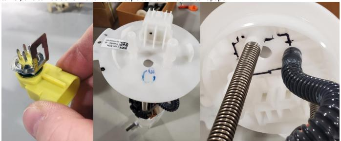
12 – The factory fuel pump power and ground wires can be removed or covered so they will not short on the module. Attach the supplied Brushless pump harness to the bulkhead and the DW440 pump.
