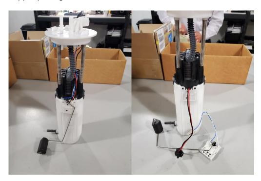
2 – Separate the bucket from the center section by unlatching the clips around the edge of the bucket. Slide the module apart and cut the factory venturi hose allowing you to fully separate the module.
