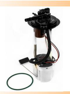
The DW400 14-18 GM Truck Module is a complete drop in replacement for the OE unit. The module incorporates the DW400 pump which out flows the OE module by more than 50%. This module also integrates seamlessly with the OE wiring harness and level sender. The module also utilizes a venturi fed surge bucket for consistent fueling at low tank levels and high G conditions.
