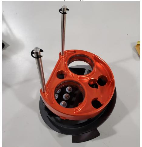
8 – Install the provided pump pre-filters onto the DW400 pumps and install the pumps into the X2 center section. Install the assembly into the bucket. Lubrication can aid in installation of the pumps. See picture for filter and pump alignment.
