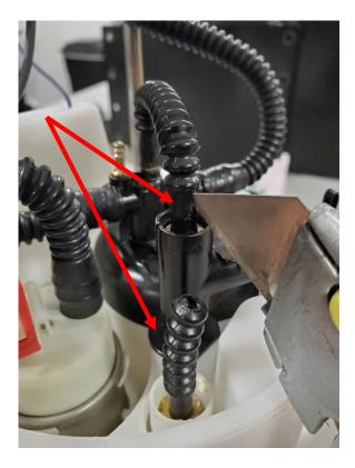
2 – Locate and pry apart the 3 lock tabs around the edge of the bucket, and separate the top hat, pump, filter and center section from the bucket assembly.
