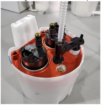
10 – Cut the supplied 12" long 3/8" ID convoluted tube down to 7" inch long and install onto the return fitting on the bottom side of the X2 top hat, secure with one of the 13.3mm pinch type hose clamp. This return hose should be routed through the hole centered at the back between the DW400 fuel pumps.
