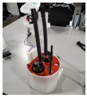
12 – Install the opposite end of the 6" long 3/8" ID hoses onto the remaining  $2x \ 3/8$ " hose barb fittings on the bottom side of the X2 top hat. The hoses should cross over to provide space for the module to compress. See picture for suggested routing.
