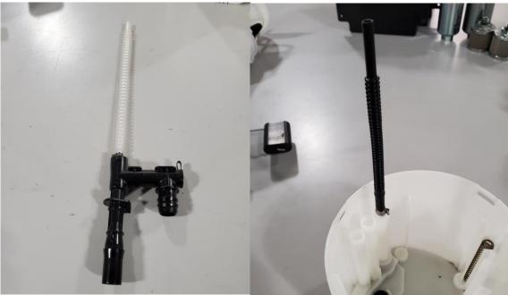
6 – Install the separate 3/8" hose barb to -6 AN O-Ring fitting into the billet X2 top hat, on the bottom side return port.
